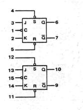
VCC = Pin 16 Gnd = Pin 8 The negative–edge–clocked dual J-K flip-flop operates on the master–slave principle. His device provides both SET and RESET inputs on both flip-flops in the package. Each flip-flop may be set or reset by applying a low level to that particular input when the clock is low.
